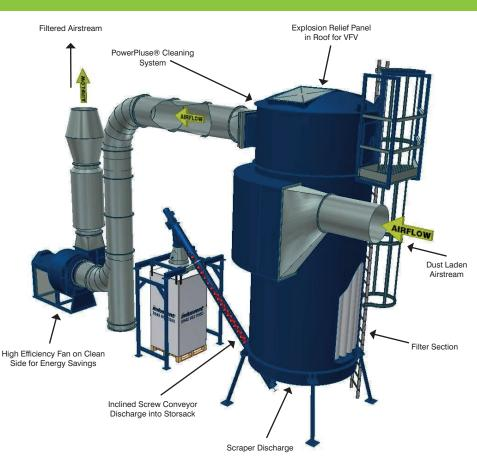
For Applications upto 45000m<sup>3</sup>/h the Super-Blower Filter is an extremely efficient negative pressure filtration system allowing 24hr operation. Manufactured from 3mm Mild Steel and Powder coating provides a strong hard wearing construction.
